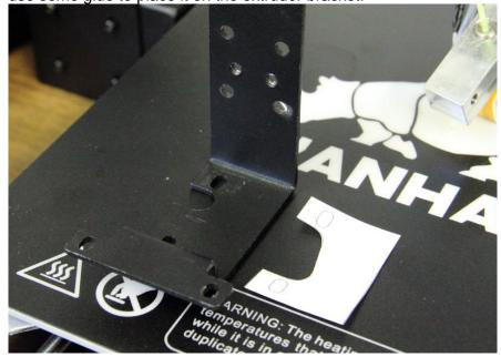
11. Attach the template to the bottom side of the bracket and align the holes printed on
