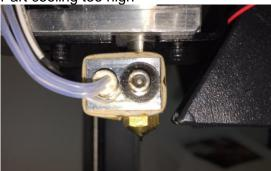
Part cooling fan at correct height
