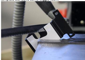
13. Use a metal file to complete the cutout. Also de-burr the edges to avoid to cut yourself when handling the part later.
